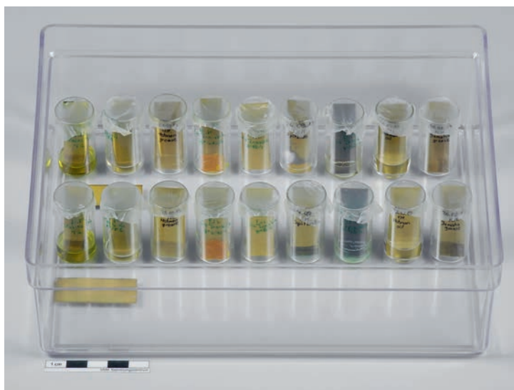
FIGURE 1 Test set-up using small brass plates to assess the corrosiveness of different oils and greases
